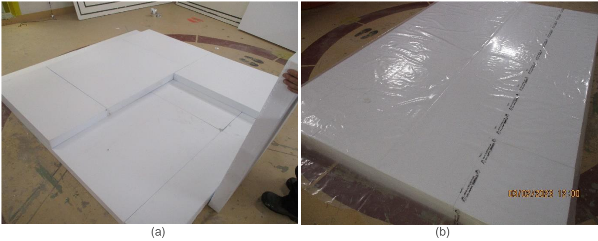
Figure 2. Preparation of the test specimen at M27 Acoustics laboratory at NRC – Rigid Insulation Layout
