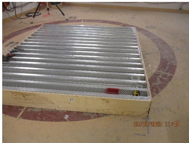
Figure 4. Assembled test specimen at M27 Acoustics laboratory at NRC. The exposed area was 6.68 m 2 .
