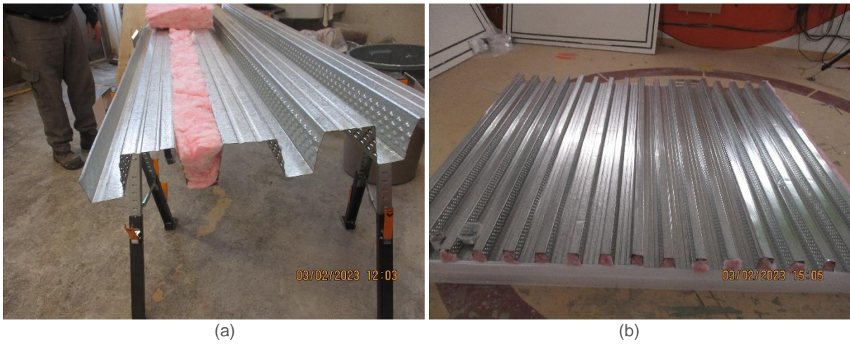
Figure 3. Preparation of the test specimen at M27 Acoustics laboratory at NRC – Steel deck Layout.
